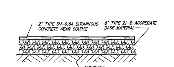
A STANDARD-DUTY BITUMINOUS PAVEMENT
