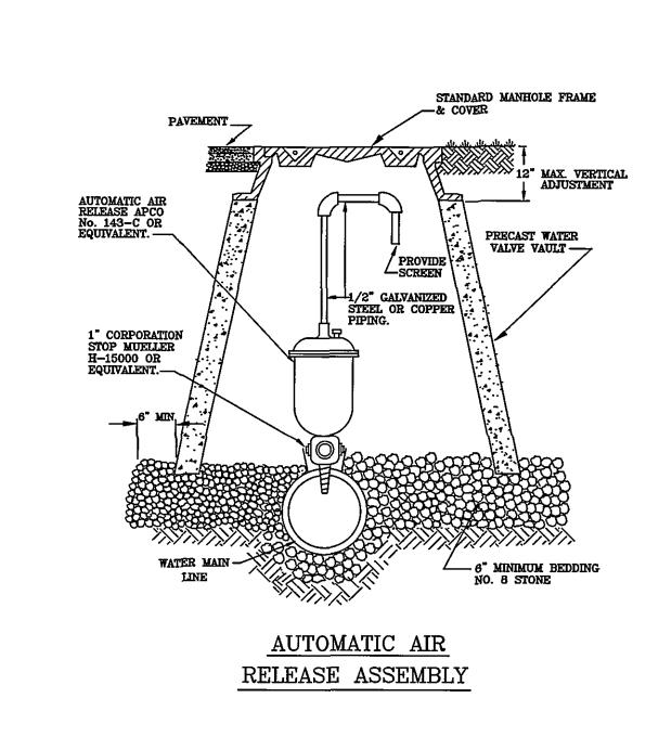
WATER LINE VALVE INSTALLATION
