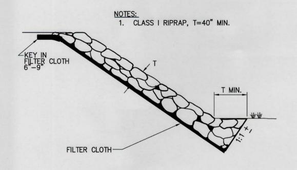
RR 3 TOE REQUIREMENTS FOR BANK STABILIZATION SCALE: N.T.S.
