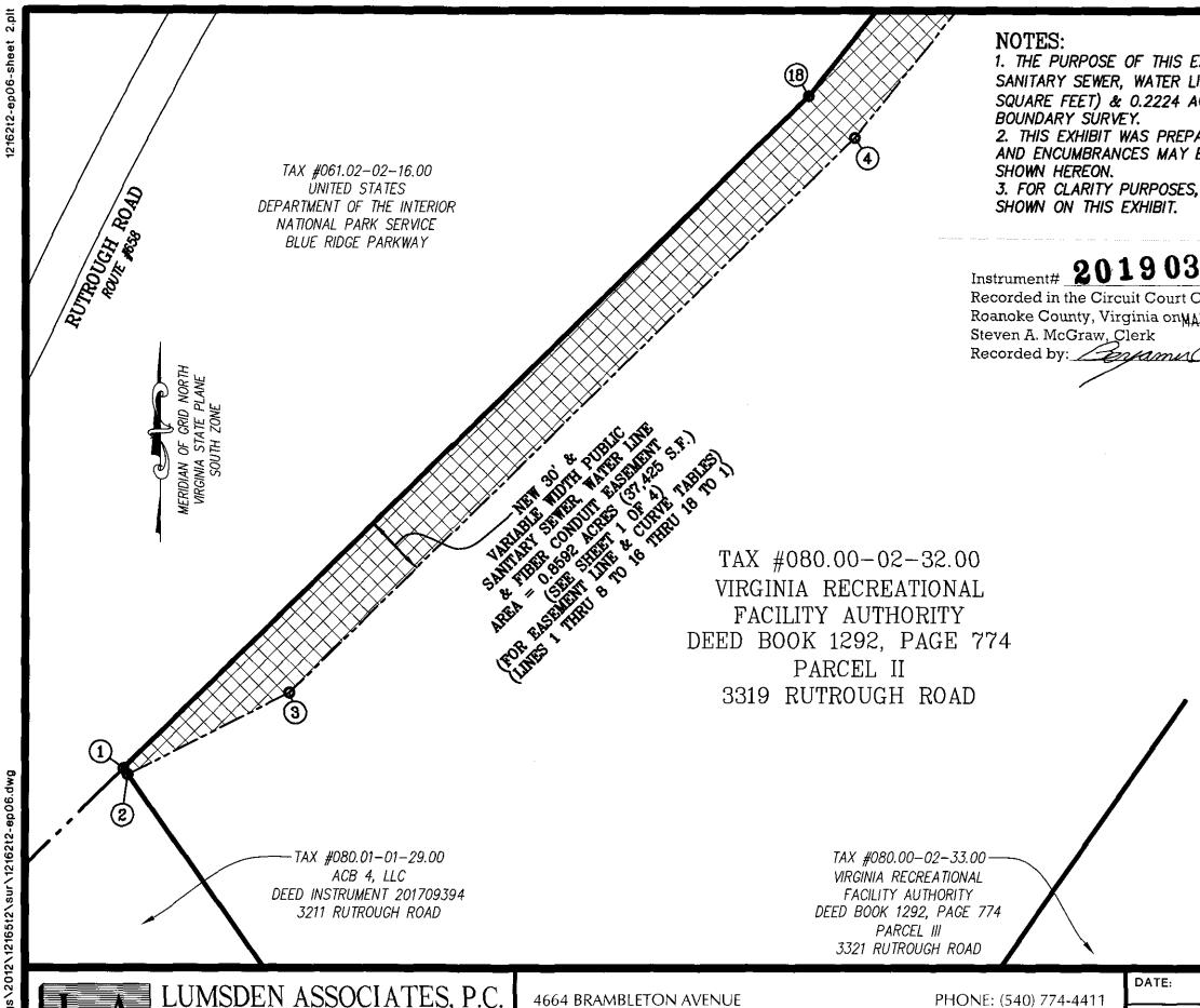
1. THE PURPOSE OF THIS EXHIBIT IS TO CREATE A NEW 30' & VARIABLE WIDTH PUBLIC SANITARY SEWER. WATER LINE & FIBER CONDUIT EASEMENT, 0.8592 ACRE (37,425 SQUARE FEET) & 0.2224 ACRE (9,688 SQUARE FEET) AND DOES NOT CONSTITUTE A BOUNDARY SURVEY.
