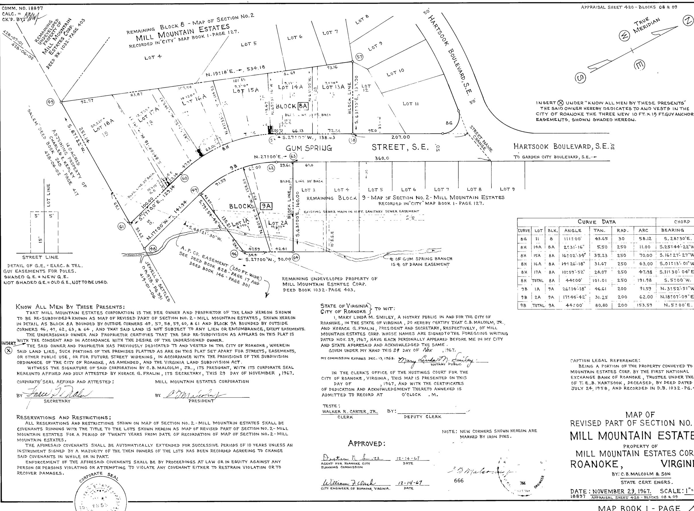
CURVE DATA CHORD ARC BEARING DIST. CURVE LOT | BLK. 43.65 30 58.12 5,28:30'E. 49.45 111200 11.00 | S.25°44'-22"W. 2231-16" 47,98 S.11:30-04"E. 47.91 24.07 101.01 250 191.98 S.5°00'W. 187.31 91.59 N. 3252'-51"W. 90.79 62.00 N.18°07-09"E. 61.75 80,80 | 200 | 153,59 N.5°00'E. | 149.84
