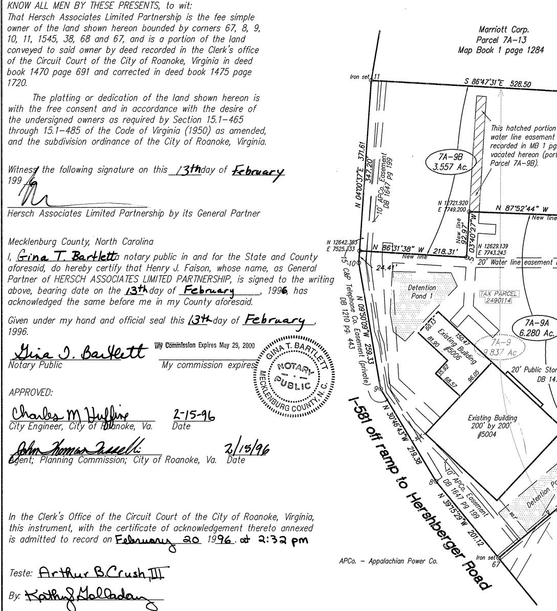
This hatched portion of the 20' water water line easement dedicated by plat recorded in MB 1 pg. 1148 is vacated hereon (portion crossing N 87°52'44" W 317.43<sup>F, 8066.416</sup> Ze Ze 20' Water line easement DB 1656 pg 798 Valley 20' Public Storm Drain Easement DB 1471 pg. 1369 Public San. Swr. Esm't. DB 1232 pg. 75
