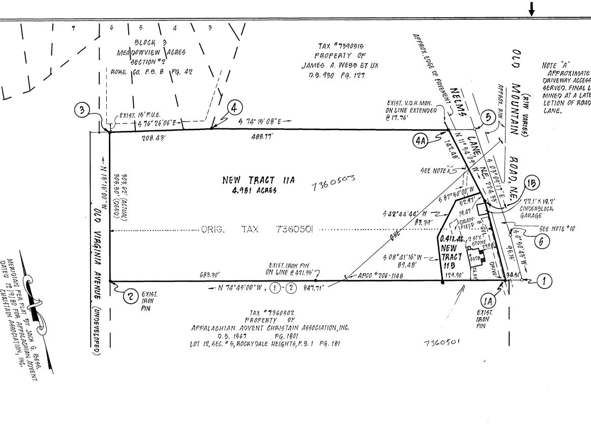
APPROXIMATE LOCATION OF PRIVATE DRIVEWAY ACCESS EASEMENT TO BE RE-GERVED. FINAL LOCATION TO BE DETER-MINED AT A LATER DATE WITH COMP-LETION OF ROAD WORK ALONG NELMS
