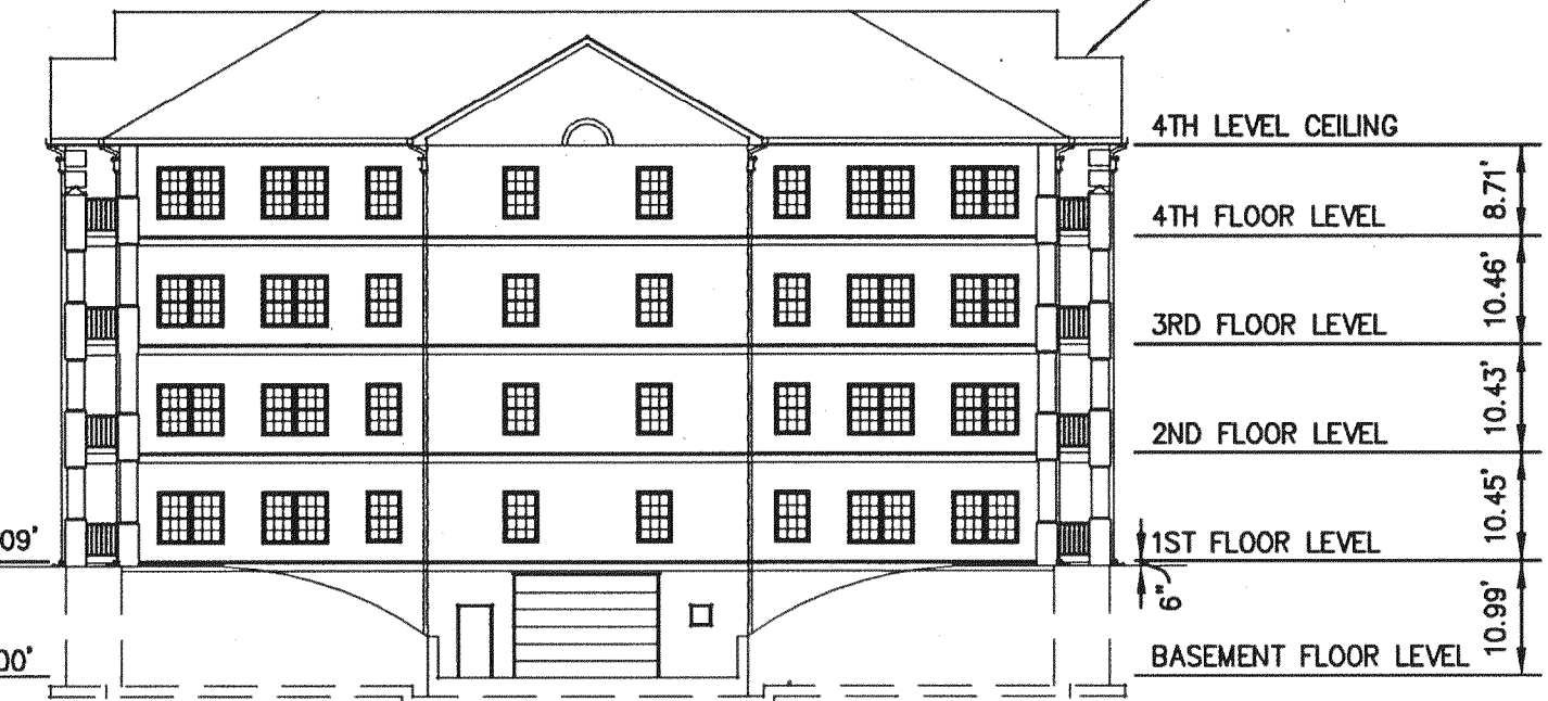
RIGHT SIDE SECTION ELEVATIONS BUILDINGS 2 & 4
