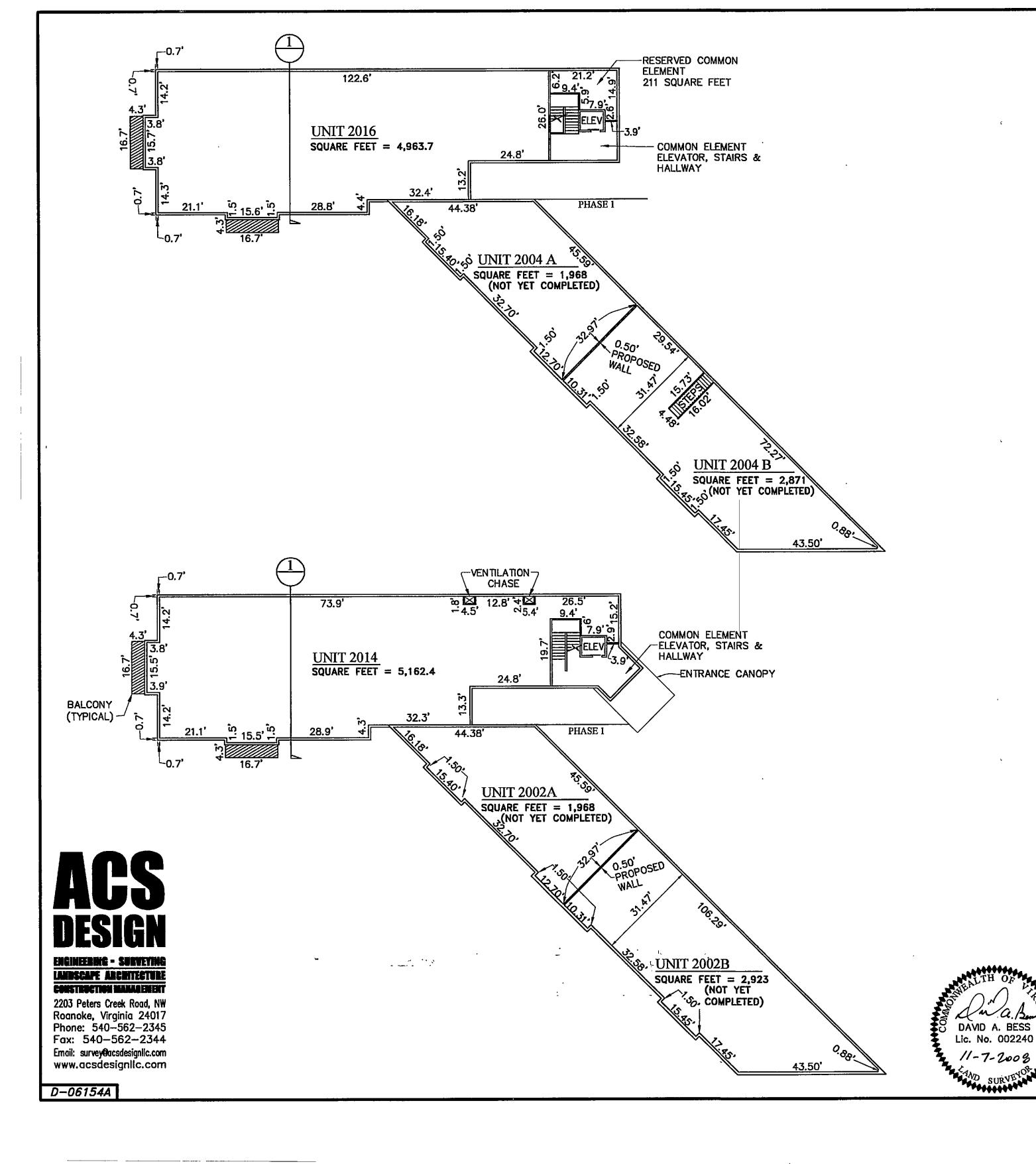
SHEET 2 OF 2 EXHIBIT "C" PLAN SHOWING LOCATION AND DIMENSIONS OF UNITS
