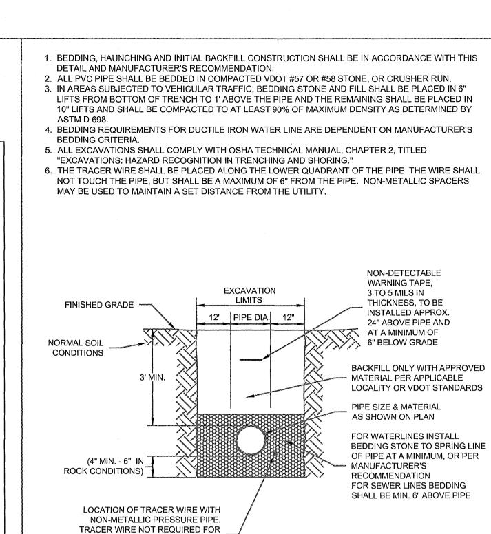
TYPICAL GRAVITY SANITARY SEWER. SEE DETAIL G-4 FOR ADDITIONAL
