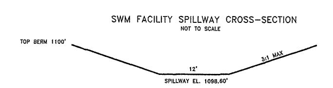
SWM FACILITY SPILLWAY CROSS-SECTION NOT TO SCALE
