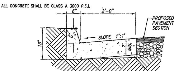
BOTTOM OF THE CURB & GUTTER -MAY BE CONSTRUCTED PARALLEL TO THE SLOPE OF THE SUBBASE
