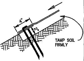
TERMINAL FOLD NOTE: BLANKET MATTING (B/M) TO BE USED ON ALL SLOPES 3:1 OR STEEPER.
