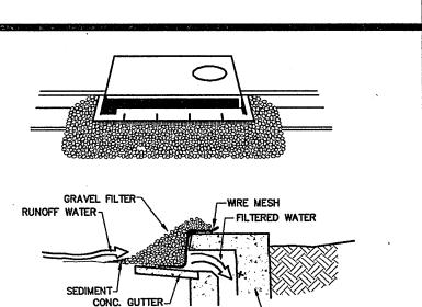
SPECIFIC APPLICATION THIS METHOD OF INLET PROTECTION IS APPLICABLE AT CURB INLETS WHERE AN OVERFLOW CAPABILITY IS NECCESSARY TO PREVENT EXCESSIVE PONDING IN FRONT OF THE STRUCTURE.
