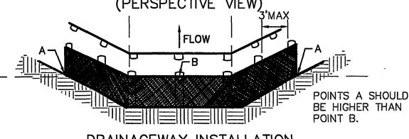
DRAINAGEWAY INSTALLATION (FRONT ELEVATION)
