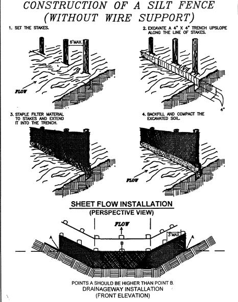
CE: Adapted from Installation of Straw and Fabric Filter Barriers for Sediment Control, VA. DSWC,
