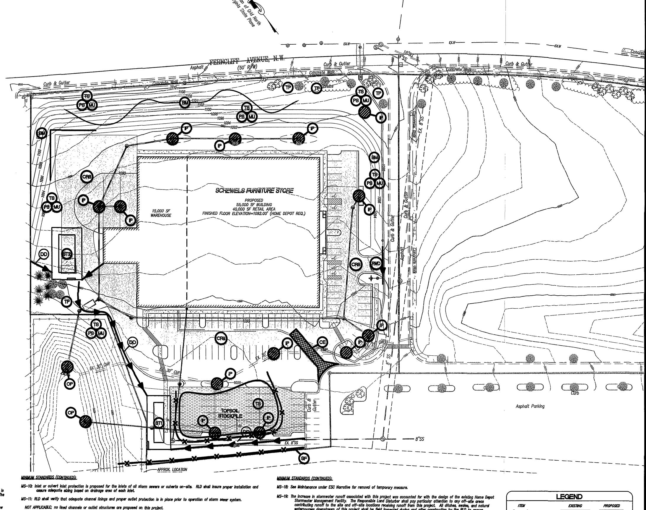
EROSION AND SEDIMENT CONTROL MEASURES FOR SITE GRADING HAVE BEEN APPROVED WITH PLANS ENTITLED 'GRADING AND EROSION CONTROL PLAND FOR SCHEWELS FURNITURE STORE," DATED FEBRUARY 7, 2007 AND ASSOCIATED WITH LAND DISTURBING PERMIT #LD070020. ADDITIONAL INLET PROTECTION IS SHOWN ON THIS PLAN TO ACCOMODATE FULL SITE DEVELOPMENT.
