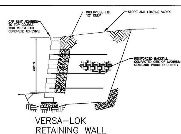
PROVIDE VERSA-LOK, ROCK WALL OR EQUAL SEGMENTED RETAINING WALL. INSTALL WALL PER MANUFACTURERS SPECIFICATIONS AND DESIGN
