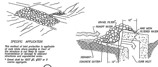
(IP) GRAVEL CURB INLET SEDIMENT FILTER
