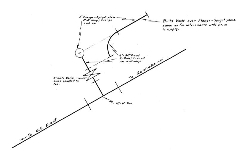
DETAILS OF BLOW OFF VALVE Located 5' W. of Catch Basin in Front of G.E. Plant
