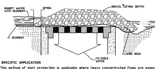
This method of inlet protection is applicable where heavy concentrated flows are expected, but not where ponding around the structure might cause excessive inconvenience or damage to adjacent structures and unprotected areas.
