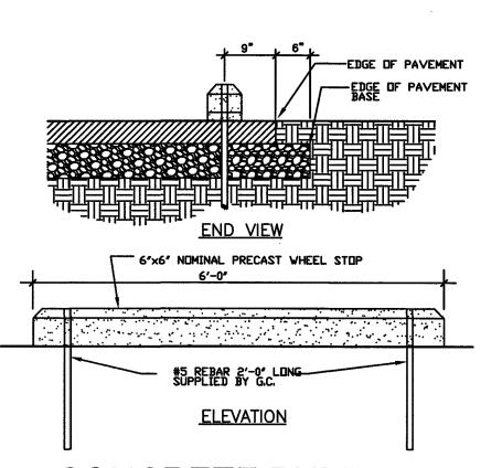
CONCRETE BUMPER BLOCK DETAIL MULTI-STEM PLANTING DETAIL
