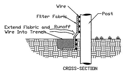
1. SET THE STAKES. 2. EXCAVATE A 4"X 4" TRENCH UPSLOPE ALONG THE LINE OF STAKES
