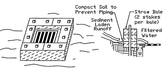
STRAW BALE DROP INLET SEDIMENT FILTER
