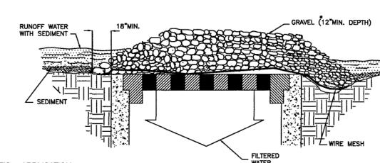
This method of inlet protection is applicable where heavy concentrated flows are expected, but not where ponding around the structure might cause excessive inconvenience or damage to adjacent structures and unprotected areas.
