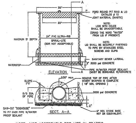
NOTE: NOT ACCEPTABLE FOR USE IN TRAFFIC AREAS OR AREAS SUBJECT TO FLOODING. SAMPLING STRUCTURE DETAIL LIST OF DRAWINGS
