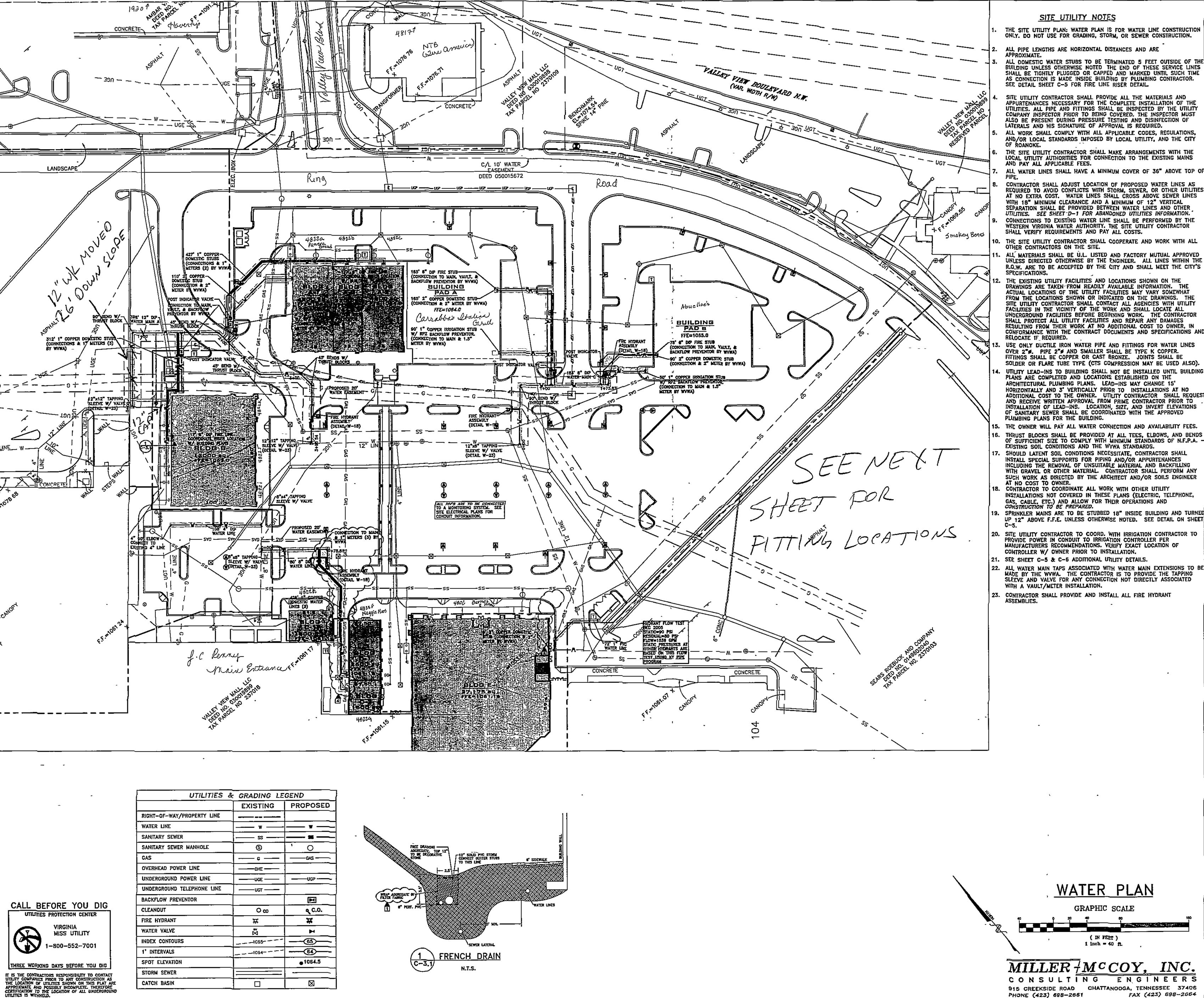
THE SITE UTILITY PLAN: WATER PLAN IS FOR WATER LINE CONSTRUCTION ONLY. DO NOT USE FOR GRADING, STORM, OR SEWER CONSTRUCTION.
