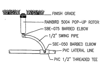
INSTALLATION DETAIL 9 4" POP-UP TURF ROTOR
