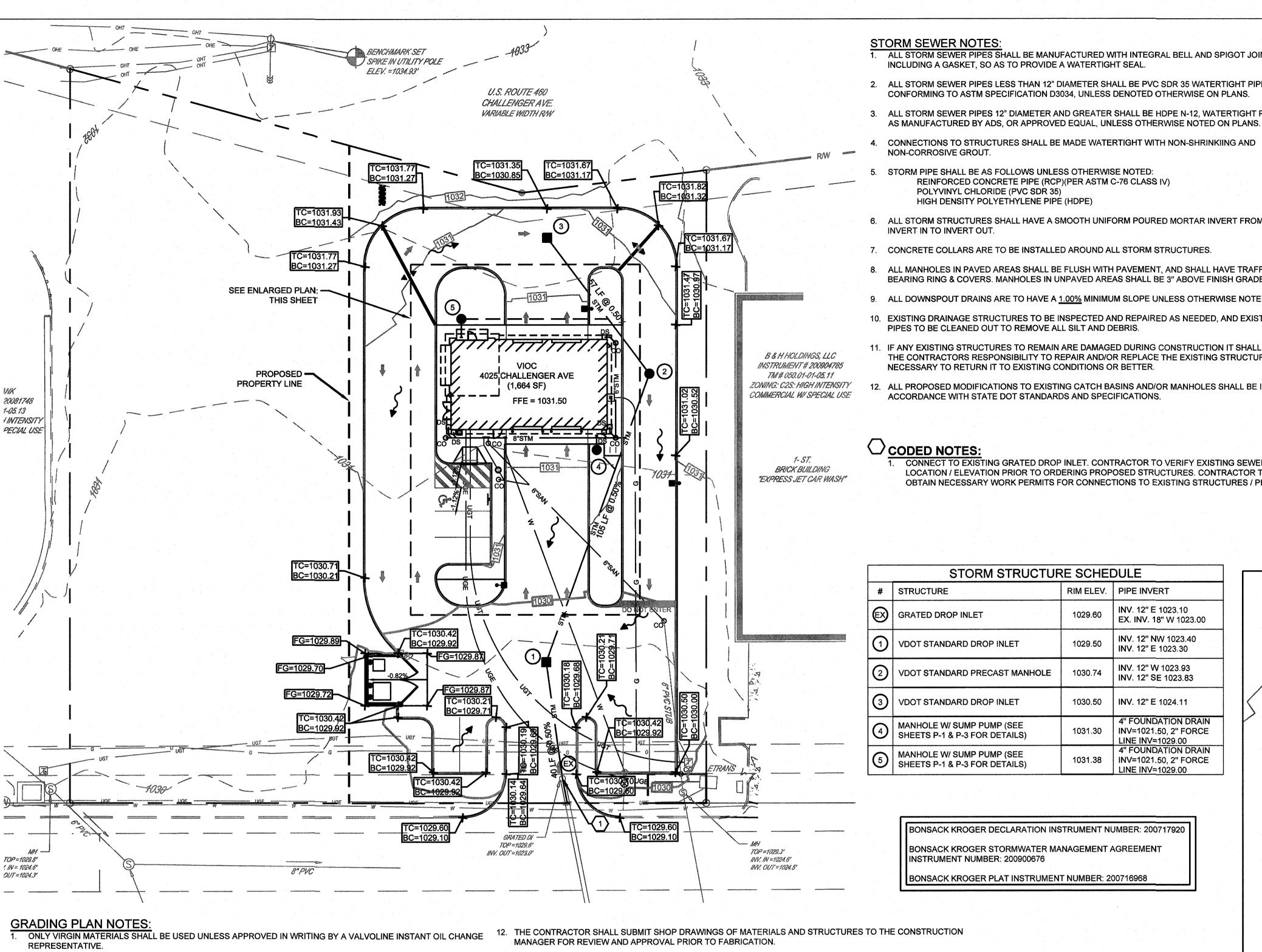
STORM SEWER NOTES: ALL STORM SEWER PIPES SHALL BE MANUFACTURED WITH INTEGRAL BELL AND SPIGOT JOINTS
