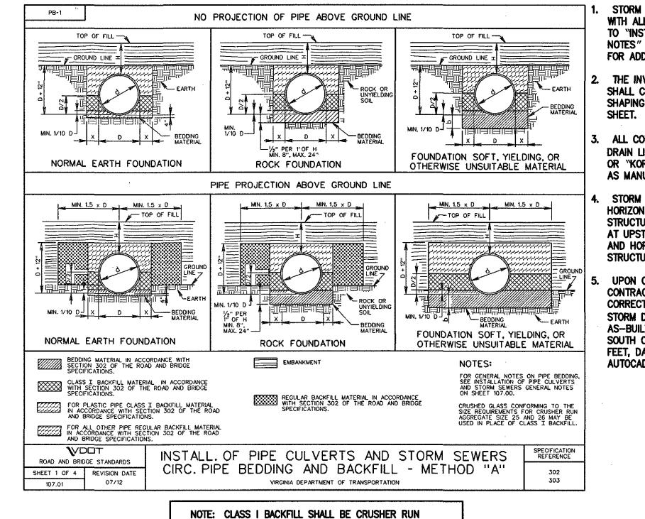
AGGREGATE SIZE NO. 25 OR 26, AGGREGATE BASE MATERIAL SIZE 21A OR 21B, FLOWABLE FILL, OR CRUSHED GLASS CONFORMING TO THE SIZE REQUIRED FOR CRUSHER RUN AGGREGATE SIZE 25 AND 26.
