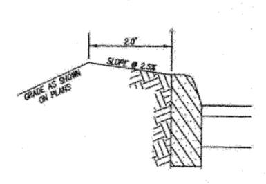
2" ASPHALT CONCRETE: TYPE SM-9.5A
