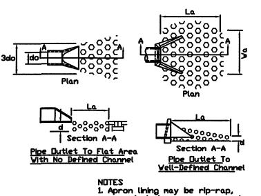
1. Apron lining may be rip-rap, grouted rip-rap, or concrete. 2. La is the length of the riprap apron as calculated using plates 1.36d and 1.36e. 3. d = 1.5 times the maximum stone diameter, but not less
