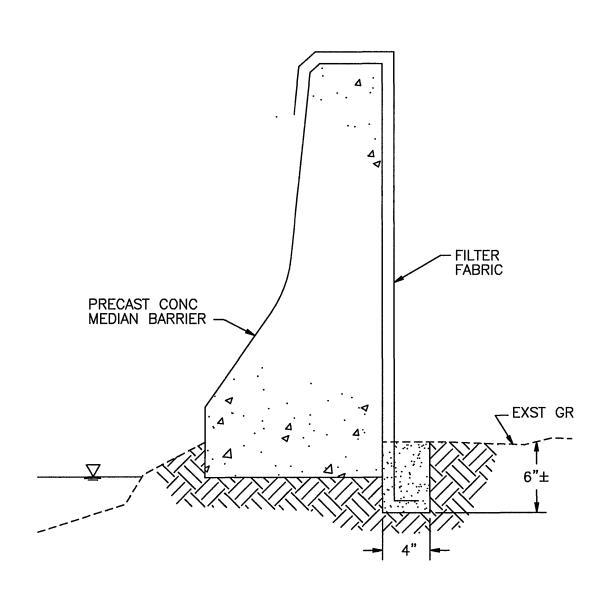
SILT FENCE CLOSE TO STREAMS SCALE:  $1 \frac{1}{2} = 1' - 0"$
