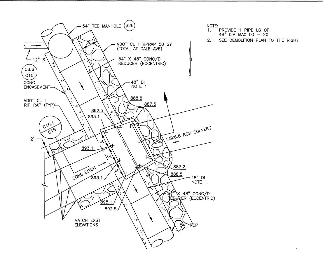
ENLARGED DETAIL SANITARY SEWER CROSSING CULVERT AT DALE AVE. SCALE: 1"=5"
