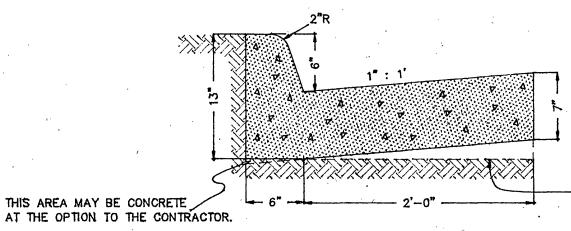
THE BOTTOM OF THE CURB, AND GUTTER MAY BE CONSTRUCTED PARALLEL TO THE SLOPE OF SUB-SURFACE COURSES PROVIDED A MINIMUM DEPTH OF 7" IS MAINTAINED.
