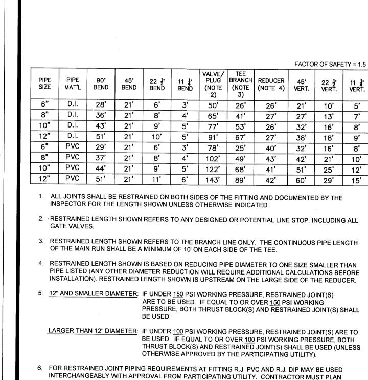
ACCORDINGLY FOR THE DIFFERENCE IN PVC AND DIP BELL AND SPIGOT DIMENSIONS.
