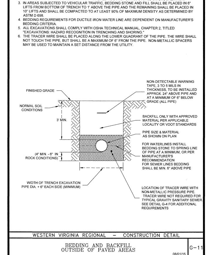
BEDDING, HAUNCHING AND INITIAL BACKFILL CONSTRUCTION SHALL BE IN ACCORDANCE WITH THIS
