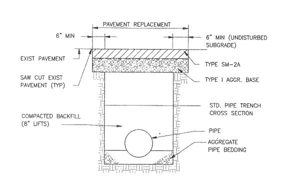
PAVEMENT REPLACEMENT DETAIL NO SCALE
