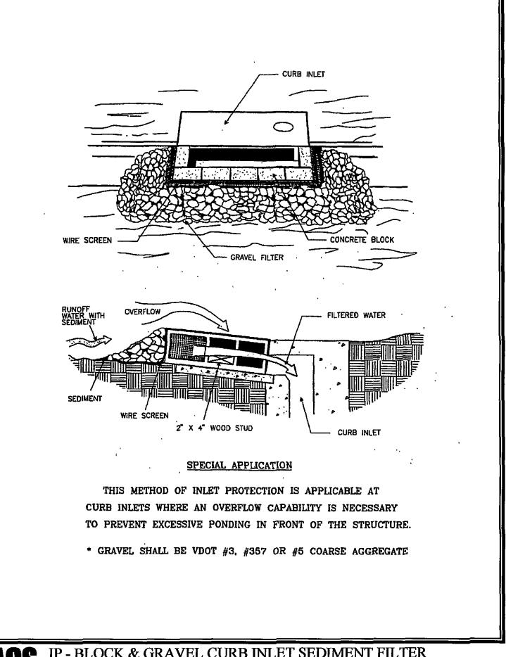
IP - BLOCK & GRAVEL CURB INLET SEDIMENT FILTER 2203 PETERS CREEK ROAD, NW - ROANOKE, VIRGINIA 24017 - Phone 540.562 2345 - Fax 540.562.2344
