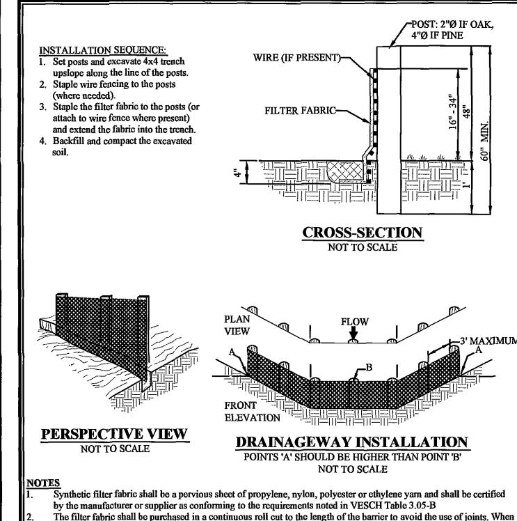
joints are unavoidable, filter cloth shall be spliced together only at a support post, with a minimum 6-inch overlap, and securely sealed. A trench shall be excavated approximately 4-inches wide and 4-inches deep on the upslope side of the proposed
