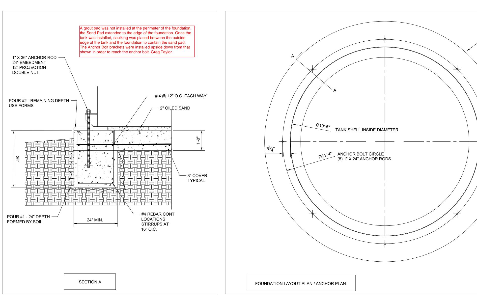
NOTE: PER GEOTECHNICS SUBSURFACE INVESTIGATION REPORT, FOUNDATION SITE SHALL BE UNDERCUT BY 6'-0" AND BACKFILLED WITH COMPACTED SELECT FILL (VDOT NO. 21A CRUSHED STONE, PLACED IN 8" HORIZONTAL LIFTS COMPACTED TO AT LEAST 95% OF STANDARD PROCTOR) TO ACHIEVE A MINIMUM 2000 PSF ALLOWABLE BEARING.
