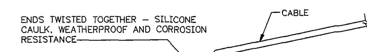
THERMOCOUPLE WIRE DETAIL NOT TO SCALE
