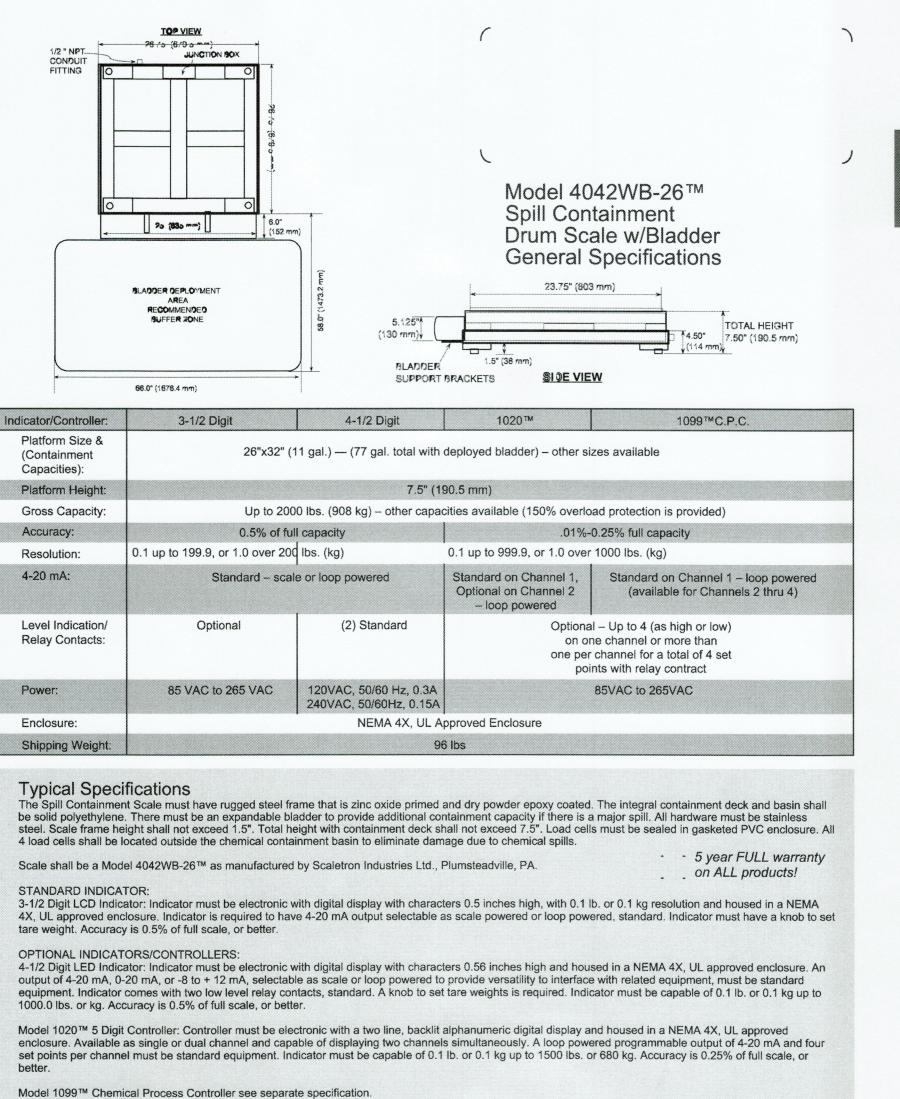
SCALETRON DRUM SCALE & CONTAINMENT
