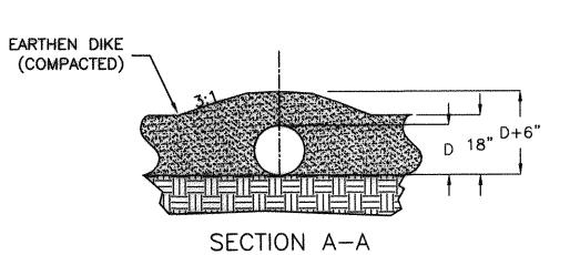
TEMPORARY SLOPE DRAIN
