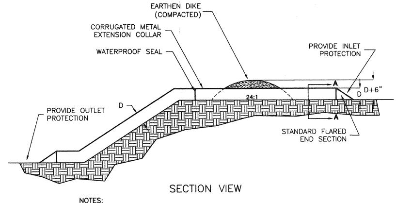
1. SEDIMENT MAY BE CONTROLLED AT OUTLET IF UPLAND PONDING WILL CREATE PROBLEMS. 2. PIPE DIAMETER SHALL BE 21".
