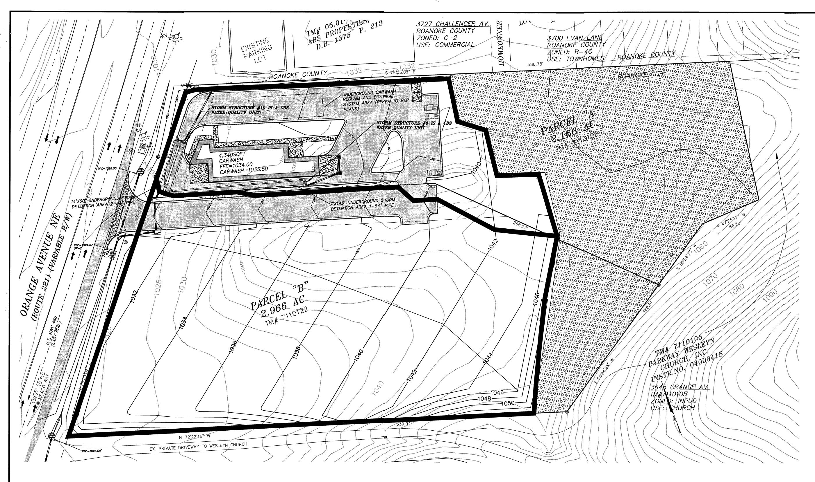
PARCEL A IS TREATING WATER QUALITY FOR THE DEVELOPMENT AS SHOWN FOR BOTH PARCELS. TWO CDS UNITS (STRUCTURE 6 AND 10) TREAT THE RECEIVED RUNOFF PRIOR TO ENTRY INTO THE UNDERGROUND DETENTION SYSTEM. THE REMAINING QUALITY TREATMENT IS OFFSITE VIA THE PURCHASE OF NUTRIENT CREDITS FROM THE ROANOKE RIVER BASIN NUTRIENT CREDIT BANK.
