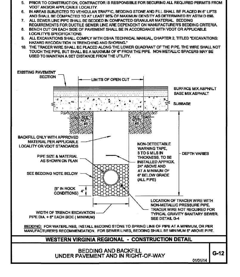
ALL PVC PIPE SHALL BE BEDDED IN COMPACTED VDOT #57 OR #58 STONE.
