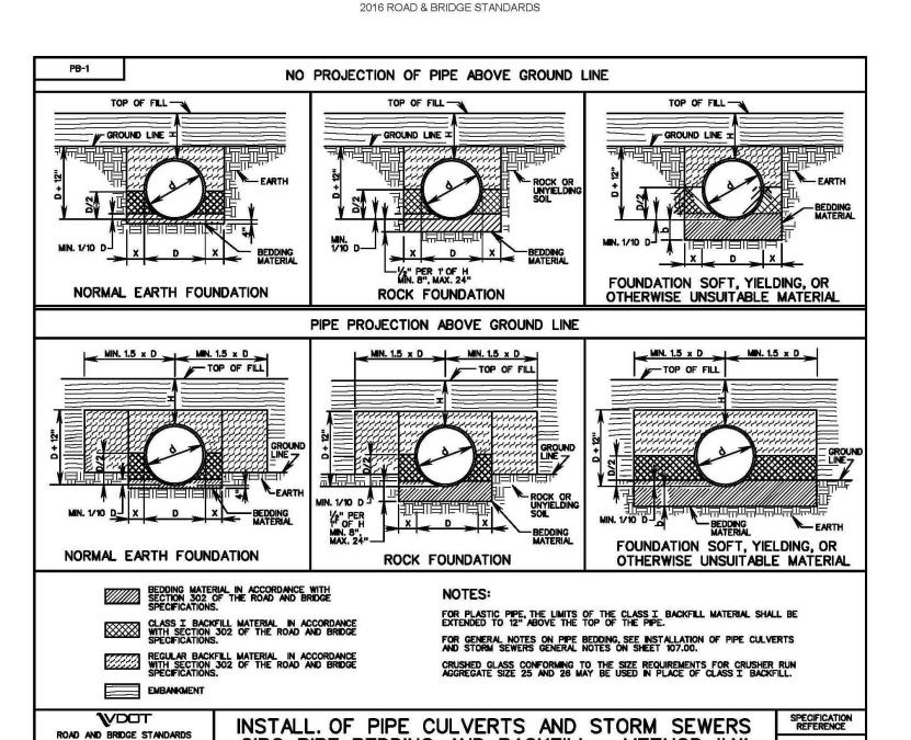
CIRC. PIPE BEDDING AND BACKFILL - METHOD "A"
