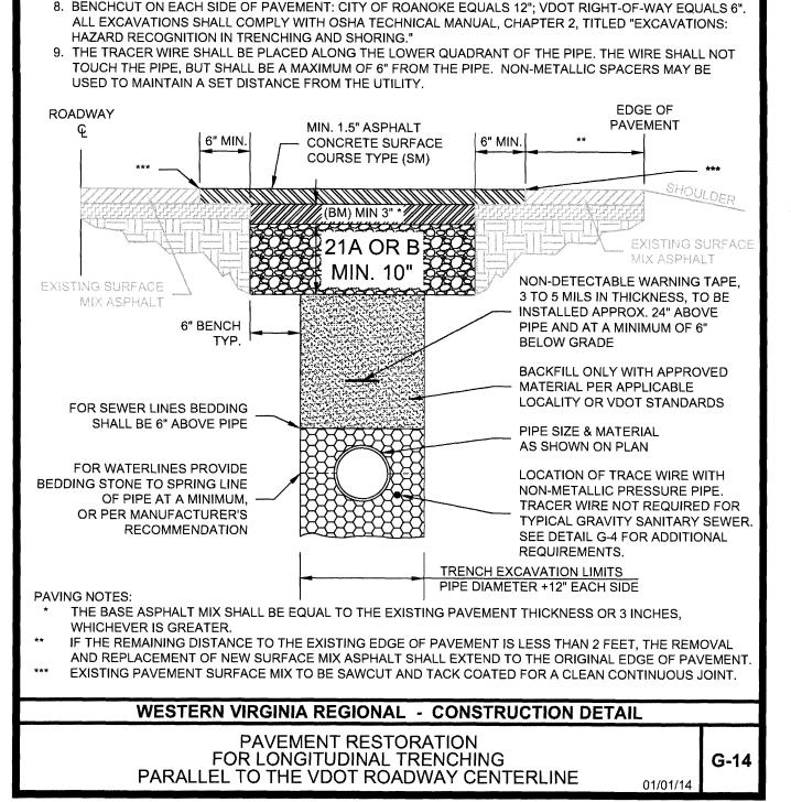
4. ALL CONSTRUCTION WITHIN THE PUBLIC RIGHT-OF-WAY SHALL BE AS SPECIFIED BY VDOT OR APPLICABLE
