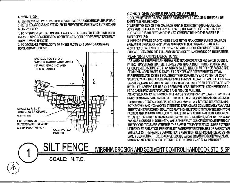
CONDITIONS WHERE PRACTICE APPLIES: BELOW DISTURBED AREAS WHERE EROSION WOULD OCCUR IN THE FORM OF 2. WHERE THE SIZE OF THE DRAINAGE AREA IS NO MORE THAN ONE QUARTER ACRE PER 100 FEET OF SILT FENCE LENGTH; THE MAX. SLOPE LENGTH BEHIND THE BARRIER IS 100 FEET: AND THE MAX, GRADIENT BEHIND THE BARRIER IS
