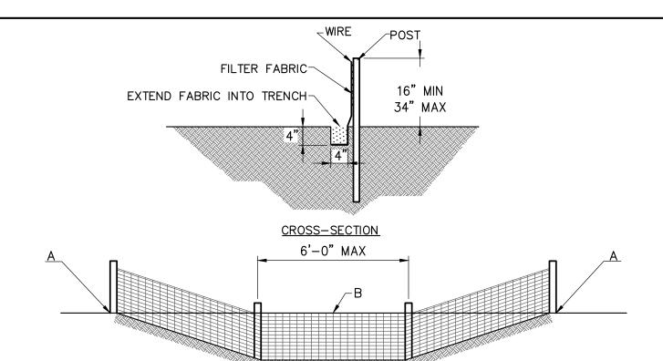
1. WHEN POINT B DROPS BELOW POINT A, USE EXTRA STRENGTH FILTER FABRIC WITH A MAXIMUM 3 FOOT SPACING OF POST.
