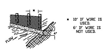
(SF) CONSTRUCTION OF A SILT FENCE
