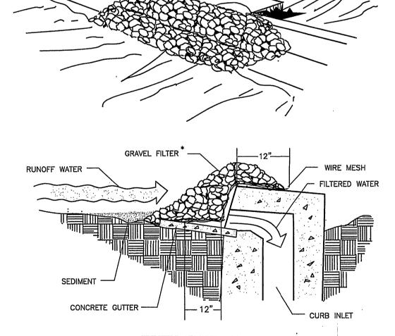
GRAVEL SHALL BE VDOT #3, #357 OR 5 COARSE AGGREGATE.
