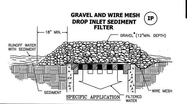
THIS METHOD OF INLET PROTECTION IS APPLICABLE WHERE HEAVY CONCENTRATED FLOWS ARE EXPECTED BUT NOT WHERE PONDING AROUND THE STRUCTURE MIGHT CAUSE EXCESSIVE INCONVENIENCE OR DAMAGE TO ADJACENT STRUCTURES AND UNPROTECTED AREAS.
