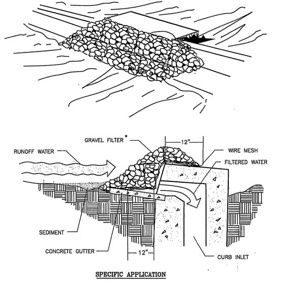
THIS METHOD OF INLET PROTECTION IS APPLICABLE AT CURB INLETS WHERE PONDING IN FRONT OF THE STRUCTURE IS NOT LIKELY TO CAUSE INCONVENIENCE OR DAMAGE TO ADJACENT STRUCTURES AND UNPROTECTED
