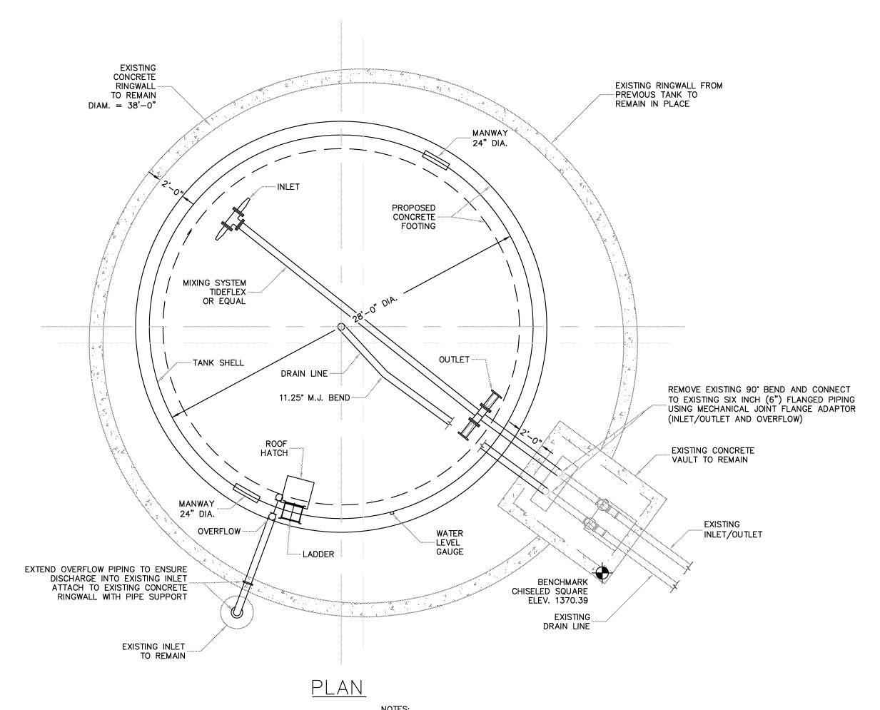
1. CONTRACTOR TO FURNISH AND INSTALL ALL MATERIAL REQUIRED TO CONNECT TO EXISTING INLET/OUTLET PIPING AND DRAIN LINE AND EXTEND PIPING TO PROPOSED TANK. ALL EXCAVATION BACKFILL AND COMPACTION SHALL BE PERFORMED BY CONTRACTOR. EXISTING CONCRETE VAULT SHALL BE SAW CUT BY CONTRACTOR AS NECESSARY TO EXTEND PIPING TO PROPOSED TANK.
